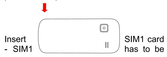
placed in the recess according to the illustration inside the phone.
