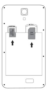
The above diagram shows the locations for Standard SIM card, battery and the Micro SD card
