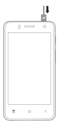
The diagram shows the correct way of inserting charger to the device.
