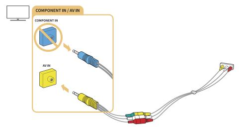
If you want to use AV (composite) equipment, remove the component adapter.
