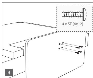
**English:** To assemble the base stand to the TV you will need a cross head screwdriver. To avoid damage to the TV screen during assembly ensure the TV is placed on a soft flat surface with the LCD screen facing downwards.
