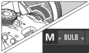
A bulb exposure keeps the shutter open for as long as you hold down the shutter button. It can be used to photograph fireworks and other subjects requiring long exposures.
