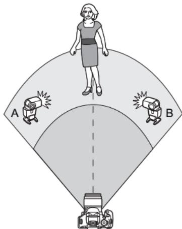
Divide the slave units into groups A and B and change the flash ratio to obtain the desired lighting effect.
