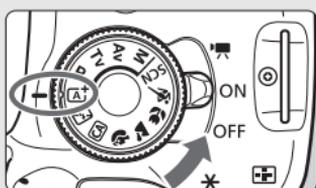
**Set the power switch to <ON>, and set the Mode Dial to <AI+> (Scene Intelligent Auto)** (p.58).
