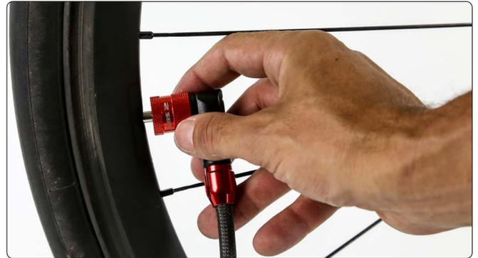
Press onto valve, slide sleeve forward and rotate sleeve 1/4 turn to seal.
