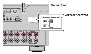
After all the connections are complete, connect the supplied power cable to the unit and then to an AC wall outlet.
