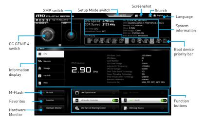
OC GENIE 4 switch - click on it to toggle the OC GENIE 4 for OC.
