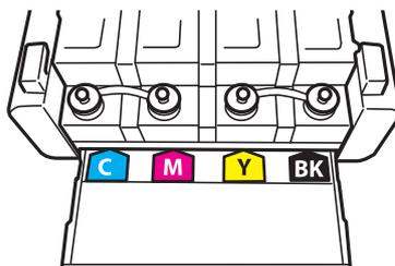
3. Snap off the top of the cap, remove the cap of the ink bottle, remove the seal from the bottle, and then install the cap.
