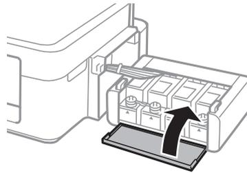
7. Hook the ink tank unit onto the printer.
