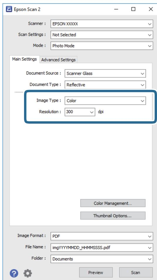
❑ **Image Type:** Select the color for saving the scanned image.
