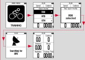
To start the training or the recording, the  $\ensuremath{\textbf{START}}$  button must be pressed once. If the stopwatch is running, it is always recorded.
