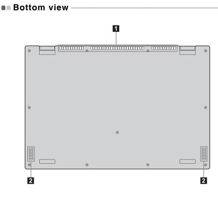
**Ventilation slots** Dissipate internal heat.
