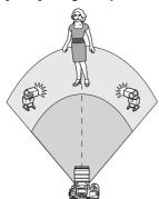
Convenient when you need a large flash output. All the slave units will fire at the same output and be controlled to obtain a standard exposure.
