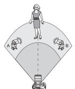
You can divide the slave units into groups A and B, and change the flash ratio to obtain the desired lighting effect. Refer to the Speedlite's instruction manual and set one slave unit to firing group A and the other to firing group B. Position the Speedlites as shown in the illustration
