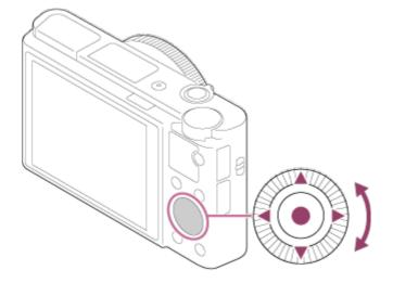
You can select setting items by turning or pressing the top/bottom/right/left side of the control wheel. Your selection is determined when you press on the center of the control wheel.
