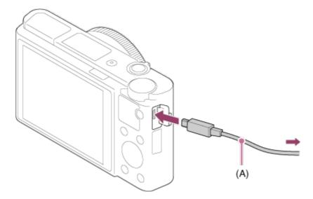
• If you connect the product to your computer using the micro USB cable wher[USB Power Supply] is set to [On], power is supplied from your computer. (Default setting: [On])
