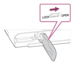
2. Insert the battery pack while pressing the lock lever(A) with the tip of the battery until the battery locks into place.
