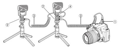
When using multiple external flashes or using an external flash with the built-in flash, P-TTL is used for flash control.
