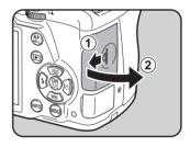
*3* Insert the card all the way with the SD Memory Card label facing toward the monitor.
