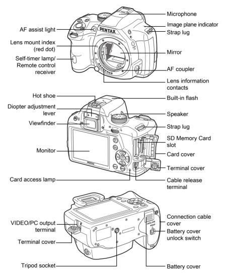
\* In the second illustration, the camera is shown with the Hot shoe cover Fκ and the Eyecup FR removed.
