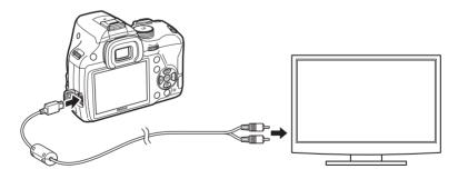
*3* Connect the other end of the cable to the input terminal on the AV device.
