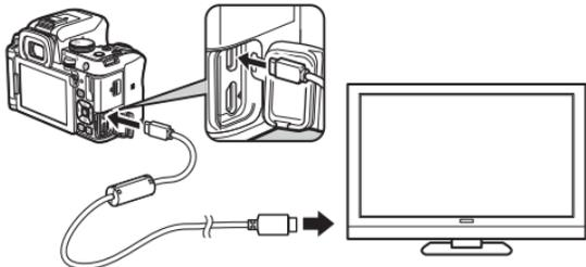
**3 Connect the other end of the cable to the input terminal on the AV device.**
