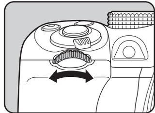
In **M** mode, the difference from the proper exposure is displayed in a bar scale while the shutter speed or aperture value is adjusted. The exposure value blinks red when the difference from the proper exposure is  $\pm 3.0$  or larger.
