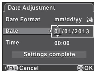
**6** Press the four-way controller (▼) to select [Settings complete], and press the **OK** button.
