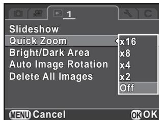
**3** Use the four-way controller (▲ ▼) to select [Bright/Dark Area] or [Auto Image Rotation], and use the four-way controller (◀ ▶) to select  or .
