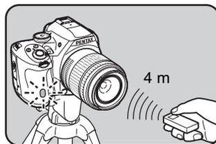
The maximum operating distance of a remote control unit is about 4 m from the front of the camera.
