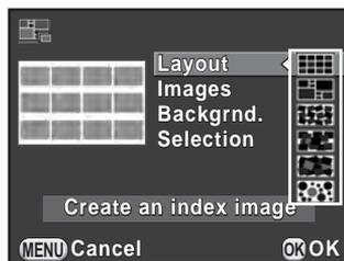
**4** Use the four-way controller (▲▼) to select [Images], and press the four-way controller (▶).
