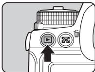
The camera enters playback mode and the most recently captured image is displayed (single image display).
