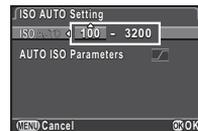
The manner in which the sensitivity is increased can be specified in [AUTO ISO Parameters].
