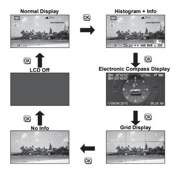
Normal Display/Histogram + Info/Grid Display in Still Picture Capture Mode 1 to 22 and A1 appear when "Normal Display" is selected. B1 to B6 appear at the
