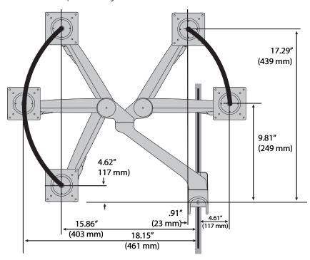
Top view showing range of motion when pulled out from the wall.
