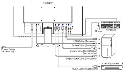
\* VGA (D-Sub) cable is not supplied with the monitor. If you use low quality VGA (D-Sub) cable, it may cause a result of electro-magnetic interference. Please contact the iiyama Support Centre in your country if you wish to connect the monitor via the VGA input.
