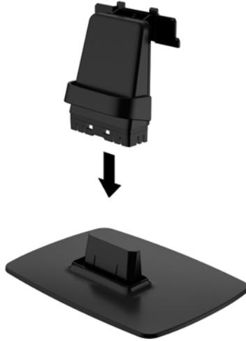
3. Insert the two tabs on the stand into the bracket on the back of the display head until they click into place.
