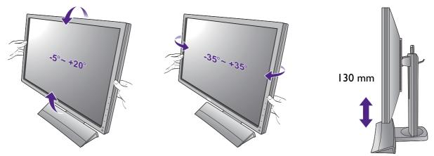
(For XL2720) You may position the screen to the desired angle with  $-5^{\circ}$  to  $+20^{\circ}$  monitor tilt, 90° (left and right total) monitor swivel, and 140 mm monitor height. XL2720
