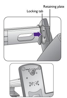
Turn the stand counterclockwise to align the arrow at the end of the stand with the one on the
