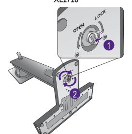
Orient and align the stand arm with the monitor
