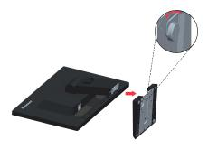
Step 4: Lift the holder up to the top point according to the figure.
