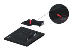
Step 6: Attach the mounting bracket from the VESA compatible wall mounting kit (100mm x100mm distance), VESA Mounting Screw M4 x 10 mm.
