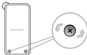
2. Replace the button battery with same type – 3V CR2032. Wait ten seconds before inserting new battery.
