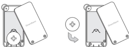
3. LED flashes red once when batteries are installed and the device is not added to your CubeOne.
