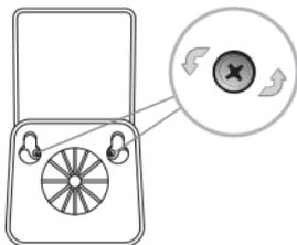
2. Replace the three AA batteries. Wait ten seconds before inserting new batteries.
