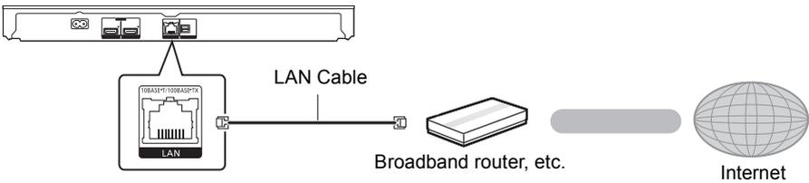
Use category 5 or above straight LAN cables (STP) when connecting to peripheral devices.
