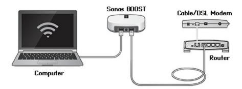
• Be sure that your cable/DSL modem is connected to the router's WAN (Internet) port.
