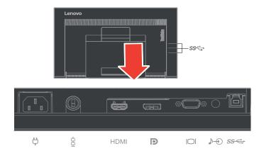
3. Connect one end of the HDMI cable to the HDMI connector on the back of the computer, and the other end to the HDMI connector on the monitor. Lenovo recommends that customers who require to use the HDMI input on their monitor purchase the "Lenovo HDMI to HDMI cable OB47070".
