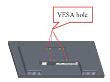
Step 5: Attach the LCD display to the wall, and follow the instructions in the wall-mounting kit.
