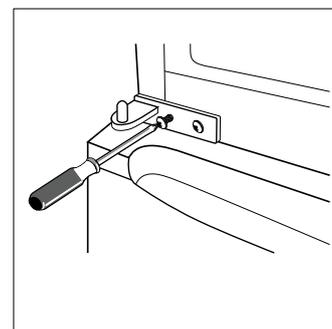
9. Place the upper door back on. Ensure the door is aligned horizontally and vertically so that the seal are closed on all sides before finally tightening the top hinge. Then insert the hinge and screw into the front of the unit.
