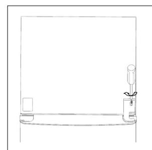
2. Unscrew and remove the hinge.
