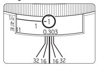
This lens enables closeup photography up to 1x magnification. The magnification is indicated by denominators above the distance scale. For example, "1" indicates "1/1x", and "5" indicates "1/5x". If you want to set the magnification first, turn the focusing ring to set the desired magnification in the manual focus mode. Then focus the subject by moving the camera forward or back.
