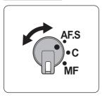
Switching the Focus Mode Change between the autofocus mode and manual focus mode at the camera. For details, refer to your camera operating manual.
