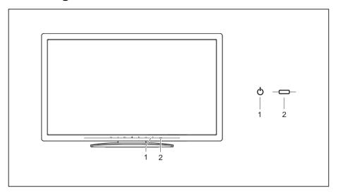
1 = Contact sensor for the on/off switch
