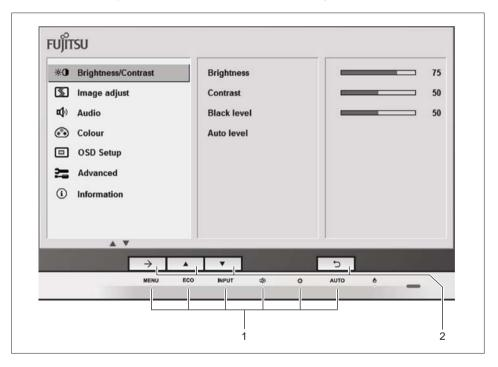
1 = Contact sensors of the control panel
