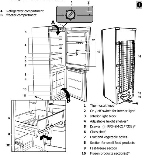
The transparent drawer **5** moves on roller bearings **22**. The drawer can be removed by pulling it out, and lifting it off the rails.
