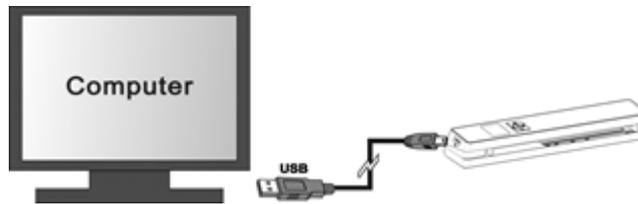
3. Press ⏻ **ENTER** briefly to enter USB mode. The USB icon is displayed on the scanner screen, and the scanner is now recognized as removable disk.
