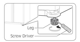
Insert a flat-blade screwdriver into a notch on the Leg, turn it clockwise or counter clockwise to level the fridge.
