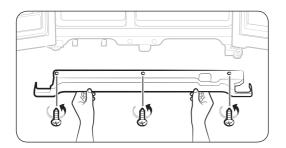
First, open both the freezer and refrigerator doors, and then take off the front leg cover by removing the three screws counter-clockwise.
