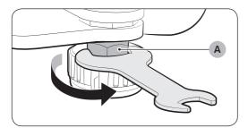
Once the doors are level, turn the clamping nut (A) counterclockwise
