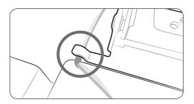
**1.** Fit the hole in the corner of the fridge door (1) over the lower hinge (2).
