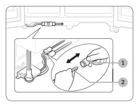
Remove the water line by pressing the coupler (1) and pulling the water line (2) away.
