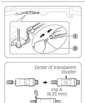
**1.** Insert the water line (2) into the coupler (1).
