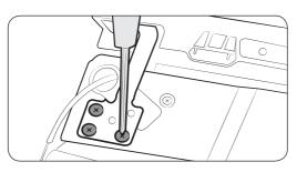
**1.** Disassemble the housing connector.
