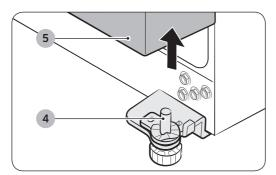
Remove the door from the lower hinge
