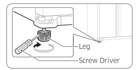
Insert a flat-blade screwdriver into a notch on the Leg, turn it clockwise or counter clockwise to level the freezer.
