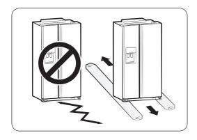
To prevent floor damage be sure the front levelling legs are in the up position (above the floor).
