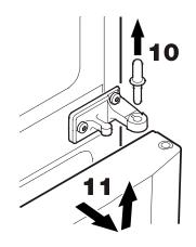
22. Transfer the hinge component on the hinge bracket to the opposite side.
