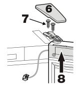
18. Remove hinge bushing, turn through 180° and re-fit.
