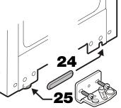
**33.** Feed in the cable of the hinge at the opposite side and insert hinge.
