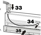
**26.** Tilt appliance slightly backwards, insert pin and attach using the adjustable foot.
