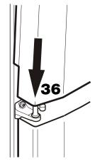
**27.** Suspend bottom door on the bottom hinge pin and close.
