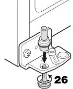
**36.** Suspend top door on middle hinge pin and close.
