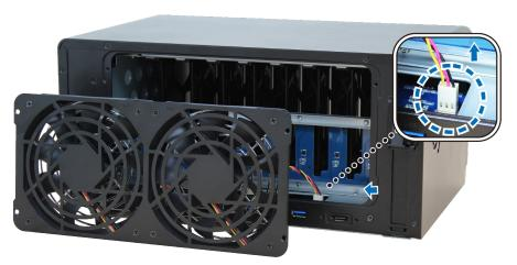
$\boldsymbol{c}\,$  Remove the 4 screws that secure the malfunctioning fan, and then remove the fan.
