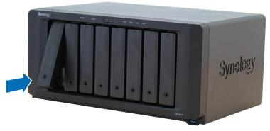
2 Pull the hard drive tray handle in the direction as indicated below to remove the hard drive tray.
