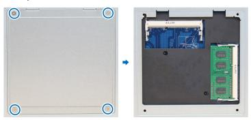
*Important:* When you remove the panel, you expose sensitive internal components. Avoid touching anything other than the memory assembly when you remove or add memory.
