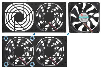
**b** Connect the 2 fan cables to the connectors located near the bottom of the fan socket, and then replace the fan panel.
