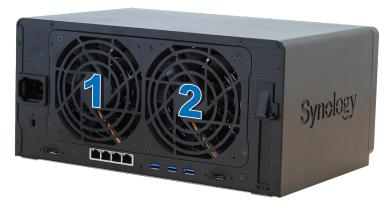
3 Remove the 4 screws that secure the fan panel.
