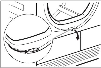
3. Turn the lever to unlock the condenser cover.
