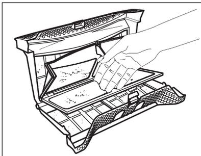
4. If necessary, clean the filter with a brush under warm tap water and/or a vacuum cleaner. Close the filter.
