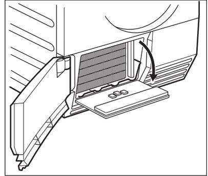
5. If necessary, remove the fluff from the heat exchanger and its compartment. You can use a wet cloth and/or a vacuum cleaner with a brush attachment.
