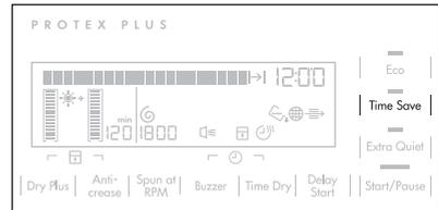
Decreases the time of the cycle without the effect on the drying quality. The cycle time can be shorter by 30% on the cottons and 40% on synthetics. The appliance operates with the higher energy consumption.
