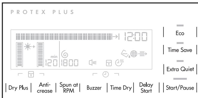
As alternative for the buttons to set the option you must touch the area with the option name. Each area between the vertical marks *senses* the user finger.
