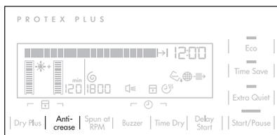
Extends of 30, 60, 90 or 120 minutes the standard anti-crease phase (30 minutes) at the end of the drying cycle. This option prevents laundry from creases. Laundry can be removed during the anti-crease phase.
