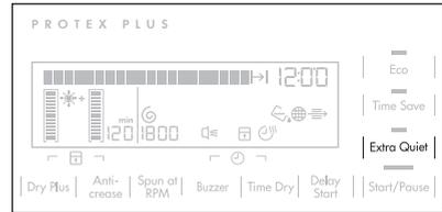
The appliance operates with low noise 62 dB without the effect on the drying quality. The appliance operates slowly with the longer cycle time.
