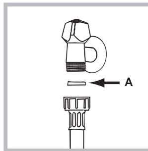
1. Insert seal A into the end of the inlet hose and screw the latter onto a cold water tap with a 3/4 gas threaded opening (see figure).
