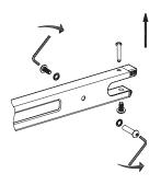
**1** Using two (2) 5 mm Allen wrenches, remove the two coupling bolts from the frame.
