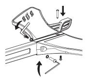
**3** Re-insert the two coupling bolts removed in Step 1. Starting underneath with the bolt on the back. Turn product over and insert the next set of bolts. Tighten using two (2) 5 mm Allen wrenches.
