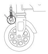
**3** If the brake is too tight or too loose, use a 8 mm wrench and a 3 mm Allen wrench to make adjustments as needed.
