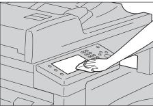
When you moisten the cloth with neutral detergent or alcohol, do not allow the excess liquid to drip down from the cloth. If the cloth is moistened with the excess liquid, wring the cloth gently before wiping the LCD area.
