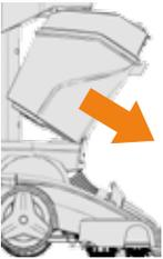
Press dirty water tank release latch, pull to remove dirty water tank.
