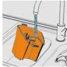
Empty dirty water over the sink. Rinse dirty water tank and lid under water to remove dirt/debris.
