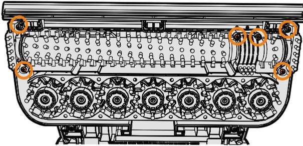
Refit belt guard and tighten x2 screws. Refit and tighten screws x2 on either side of side brushes. Refit SpinScrub brushes. Refit rug guard pins and tighten screws.
