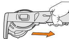
Squeeze trigger on the forward stroke, release trigger on backward stroke to recover solution/water.
