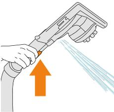
Press trigger on hose to release solution/water.
