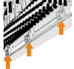
Replace nozzle by lining up tabs on nozzle with tabs underneath front of carpet washer. Push nozzle down until it clicks into place.
