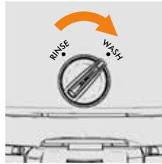
Turn wash/rinse dial to 'wash'. The SpinScrub brushes and brushbar deep clean your carpets with water and solution removing dirt and stains.
