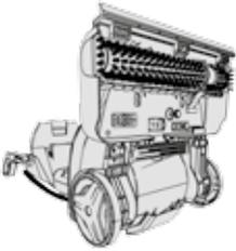
Using a pair of scissors remove any threads or hair caught around the brushbar.
