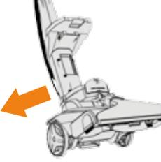
Remove both tanks and tilt carpet washer back.
