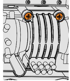
Use a crosshead screwdriver. Undo 2 screws and remove belt guard.
