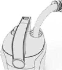
Pour required amount of carpet cleaning solution into the clean water/solution tank.
