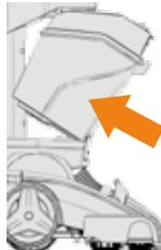
To re-fit, tilt dirty water tank and line up onto carpet washer. Push back until it clicks into place.
