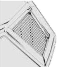
Clean the filter screen located at the back of the dirty water tank.
