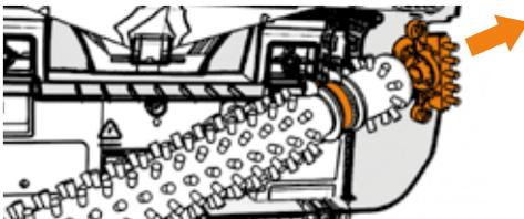
Pull and slide right side brushes together with brushbar. Remove side cap from brushbar and unloop brushbar from belt.
