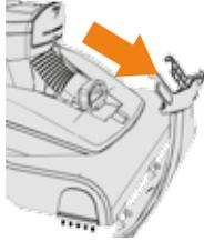
Lift nozzle release clip and pull nozzle forward, separating tabs on nozzle and carpet washer.
