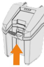
Pull and lift dirty water tank clip to release lid. Lift to remove dirty water tank lid.
