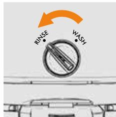
Turn wash/rinse dial to 'rinse'. Only water is released to remove solution residue.
