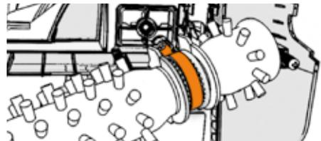
Loop replacement brushbar through belt and onto belt grip.
