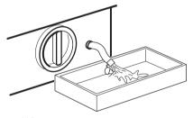
5. When no more water comes out, unscrew the pump cover (A) by turning it anti-clockwise and remove the filter. Use pliers, if necessary. Always keep a rag nearby to dry up any water spillages when removing the cover. Clean the filter under a tap, to remove any traces of fluff.
