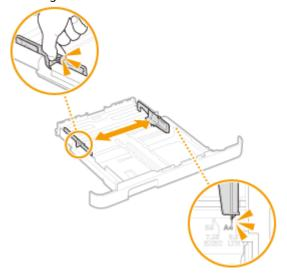
While pressing the lock release lever, move the front side paper guide to align the projection to the appropriate paper size marking.
