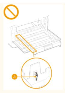
• To prevent a paper jam, do not turn OFF the power, open/close the covers, and load/unload the paper when printing.
