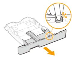
3 Load the paper so that the edge of the paper stack is aligned against the rear side of the paper drawer.
