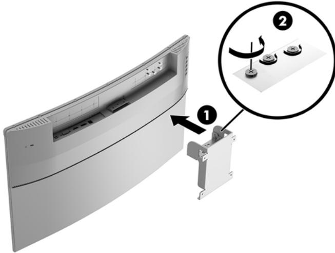
3. Secure the mounting plate to the wall or swing arm of your choice using the four screws included with the VESA mounting bracket.
