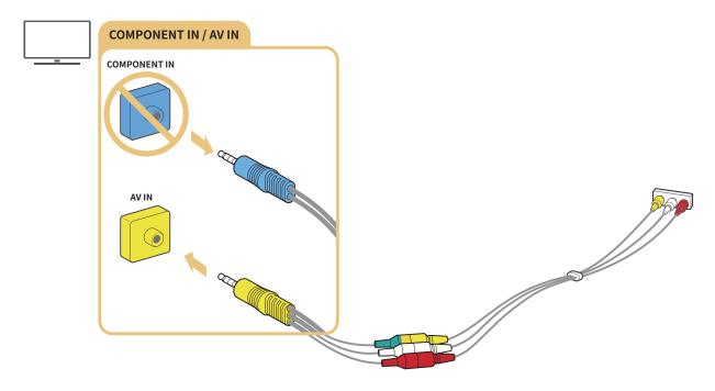
🖉 Connect AV (composite) equipment to AV In only. Do not connect to Component In.
