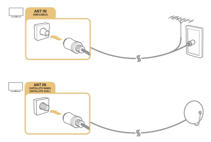
It is best to connect the both connectors using a Multi-Switch or DiSEqC. Switch, etc and to set Aerial Connection Type to Dual Oscillator.
