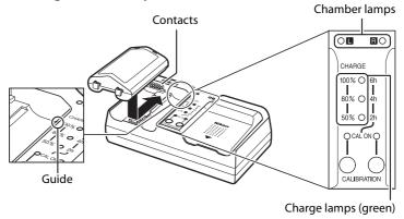
Insert the battery (terminals first), aligning the end of the battery with the guide and then sliding the battery in the direction indicated until it clicks into place. The chamber lamp and charge lamps will flash slowly while the battery charges:
