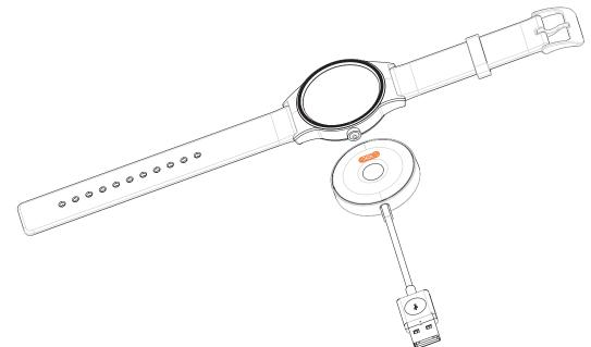
Connect the USB port with a computer to begin charging via the USB cable.
