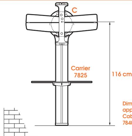
Dimensions are only applicable when Cable Column NEXT 7840 is installed.
