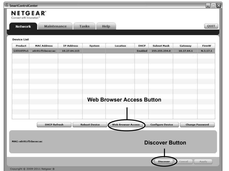
If you cannot view your switch, verify that the cable connections are secure and that the IP address configuration of the administrative computer is in the same subnet as the switch. Then click the **Discover** button.
