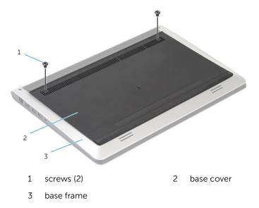
**3** Using a plastic scribe, pry the base cover off the base frame.
