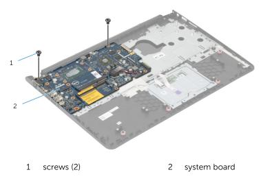
2 Lift the system board from the inner edge and release the ports from the slots on the palm rest.
